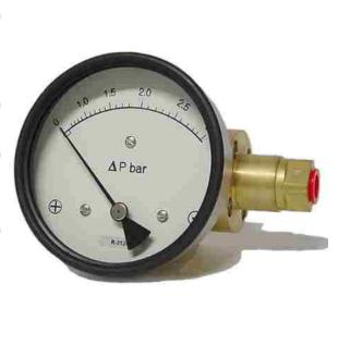
Hirlekar Precision manufactures quality differential pressure instruments designed to measure the difference in pressure between two points in a system and show it on a single dial instrument. A magnetic movement senses the differential pressure. The instruments has separate pressure and indicating chambers.
