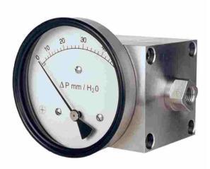
Hirlekar Precision manufactures quality differential pressure instruments designed to measure the difference in pressure between two points in a system and show it on a single dial instrument. A magnetic movement senses the differential pressure. The instruments has separate pressure and indicating chambers.
